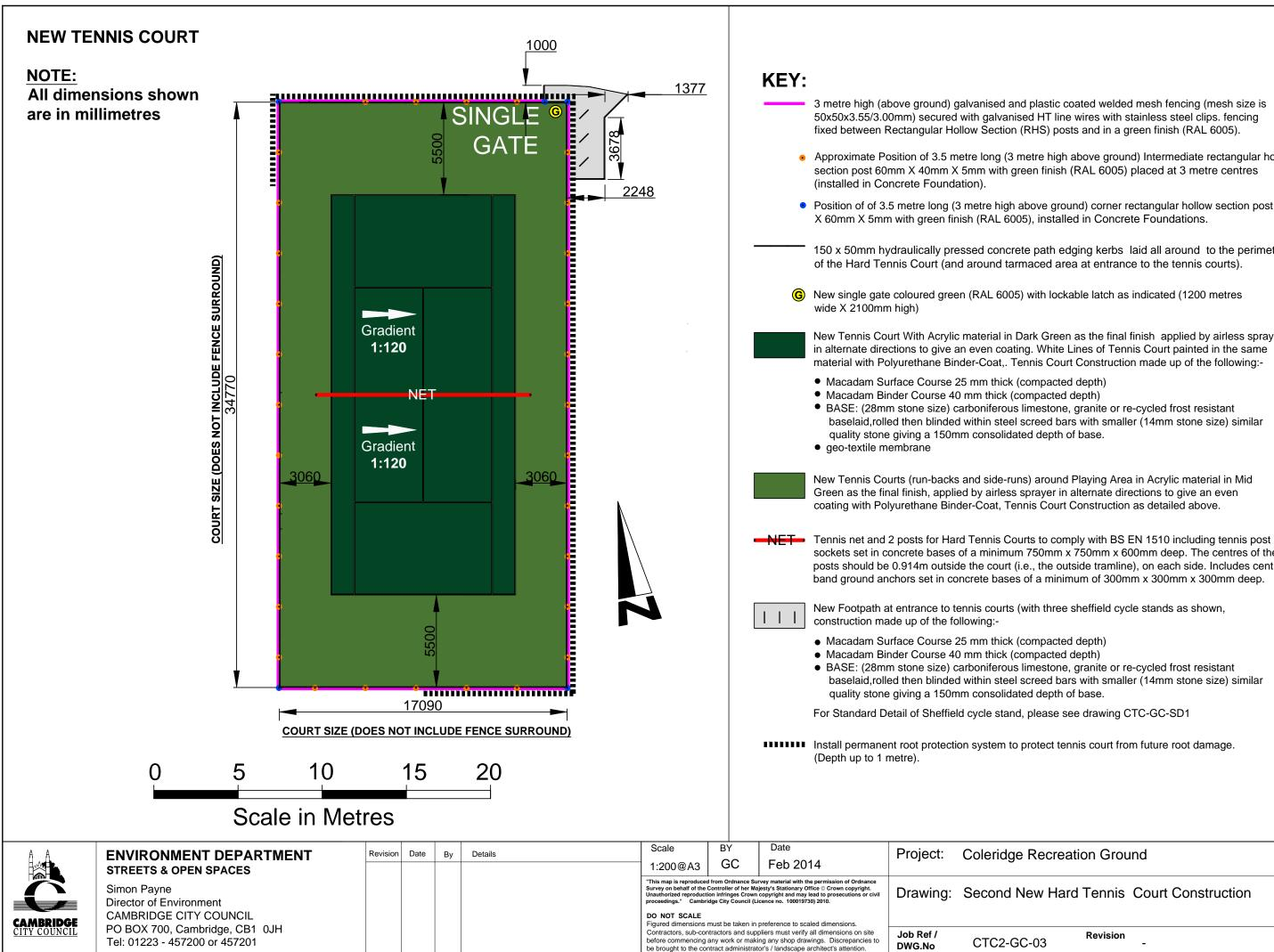
3 metre high (above ground) galvanised and plastic coated welded mesh fencing (mesh size is 50x50x3.55/3.00mm) secured with galvanised HT line wires with stainless steel clips. fencing
